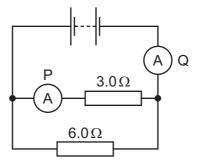
What is the combined resistance of the two resistors and which ammeter has the greater reading?
