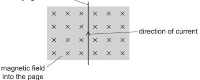
The conductor experiences a force due to the magnetic field.
